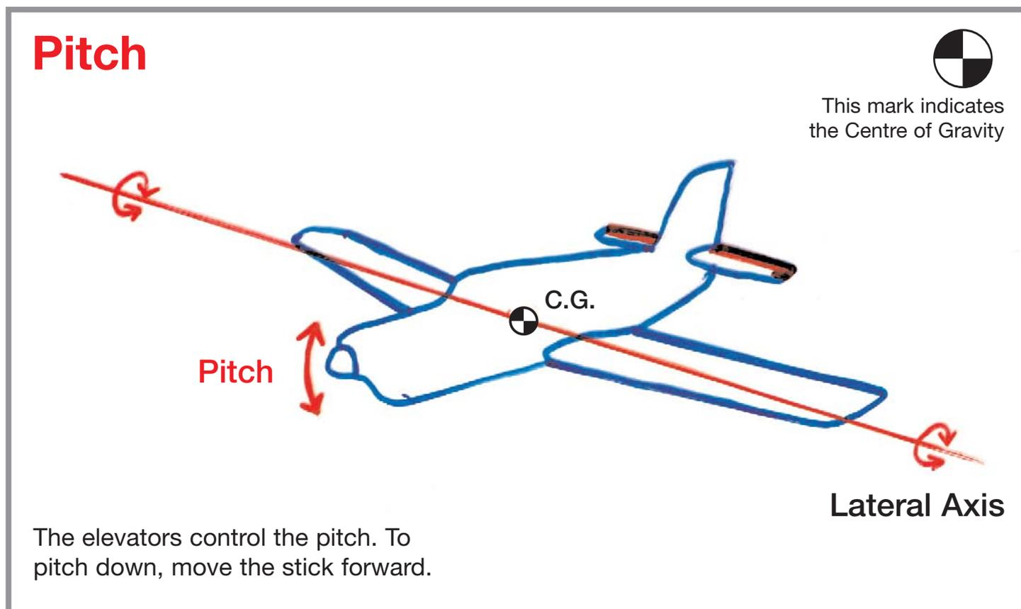
**Pitch** is the up and down movement of the aircraft’s nose around an axis line drawn from wingtip to wingtip (the lateral axis.) When you apply pitch by easing back on the stick, you angle the aircraft’s elevators up, causing the nose to rise.
