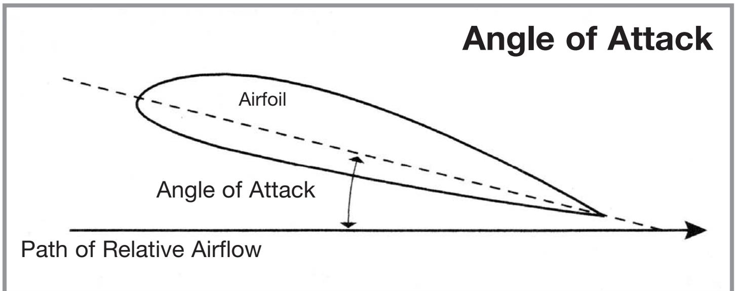
Some drag has nothing to do with air resistance, and is actually a secondary result of lift. Because lift angles backward slightly, it has both an upward vertical force and a horizontal rearward force. The rearward component is drag.
