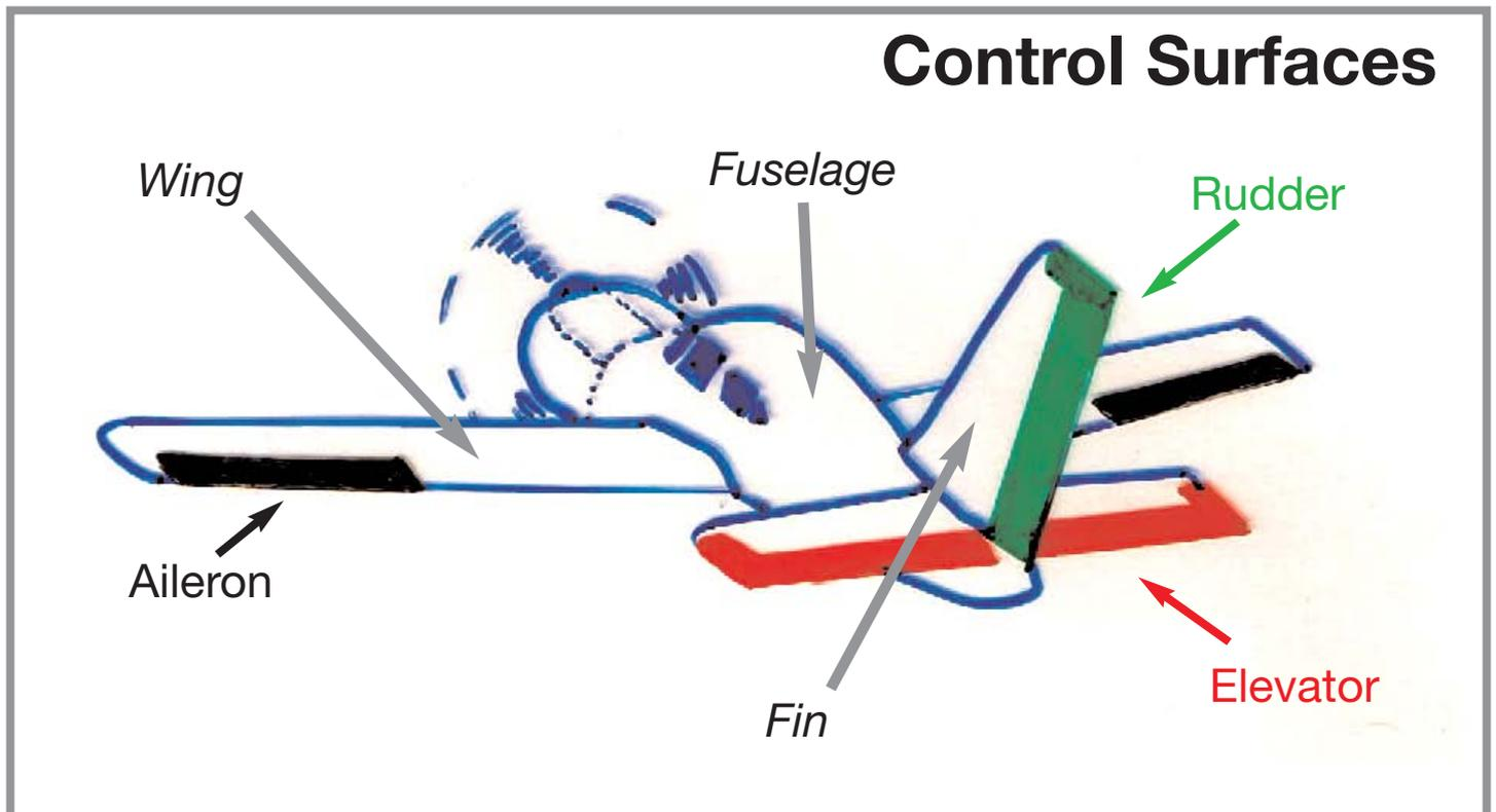
All control surfaces utilize the principles of lift, but they apply lift forces in different directions. These forces act either independently or in conjunction with one another to produce various
