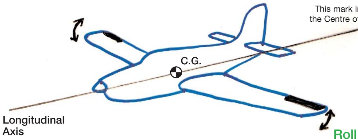
The ailerons control the roll. Move the stick to the left to roll to the left.
