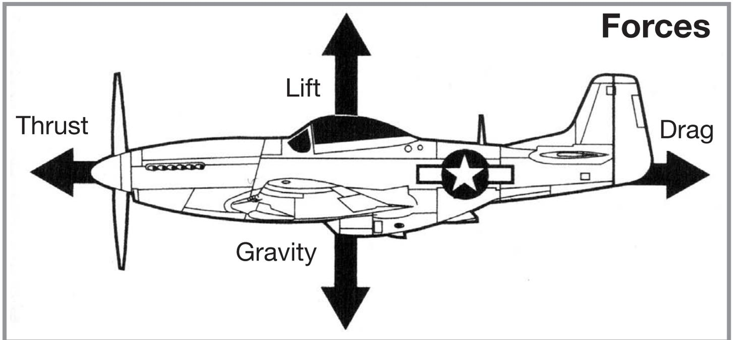
The miracle of flight exists because man has the technology to oppose natural forces that keep all objects on the ground. Four forces affect an aircraft – two assist flight (thrust and lift), and two resist flight (gravity and drag). The important thing to note here is that when an aircraft is flying straight and level, all four of these forces are balanced, or in equilibrium.
