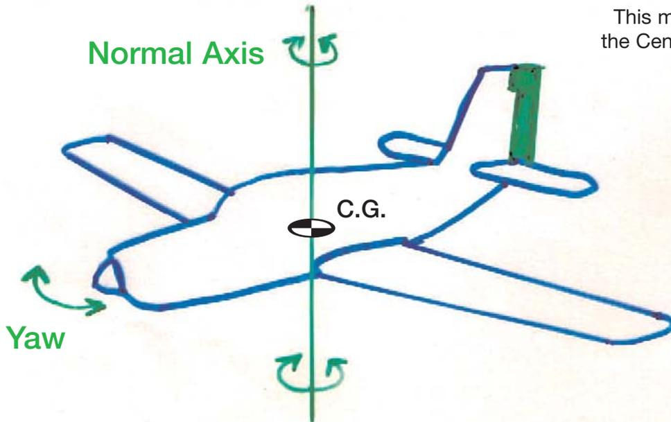
The Yaw is controlled by the rudder.
